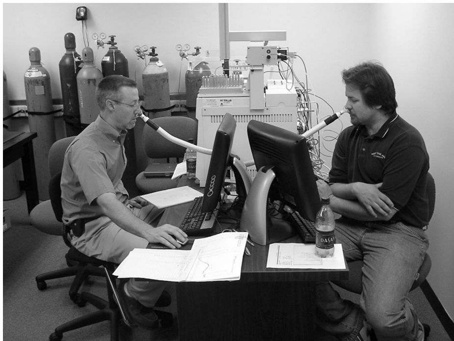
Figure 4. A gas chromatograph-mass spectrophotometer-olfactometer.
