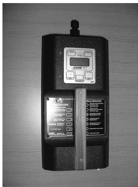
Figure 3. A Jerome meter with inlet air sampling port to the top.
