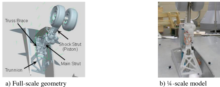
Fig. 3 Difference between full-scale and model-scale nose gear geometries at junction of main strut, trunnion, and truss brace.
