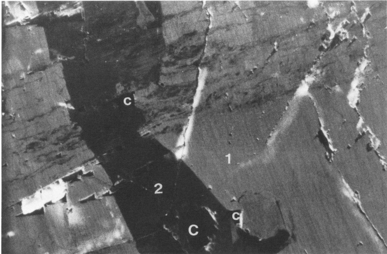
Figure 2. Photomicrograph of sample CLC-47 taken under cathodoluminescence, showing early, low-Fe calcite (moderate luminescent; zone (1), and later, high-Fe calcite (very dull luminescent; zone (2) containing fragments of coal (non-luminescent; indicated by C). Width of the field of view equals 1.25 mm.
