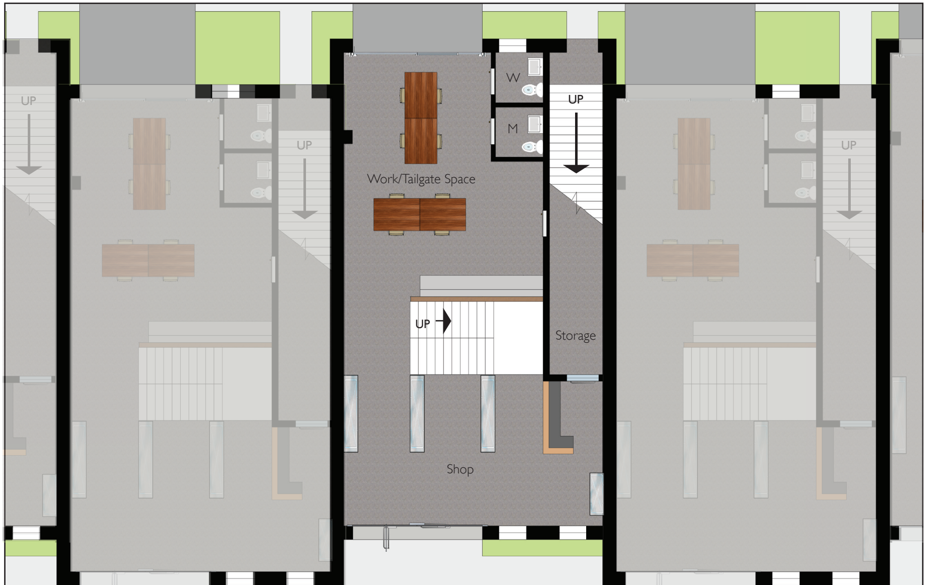
figure 5.10 Live/Work/Shop Spaces, Shop - First Floor Plan
