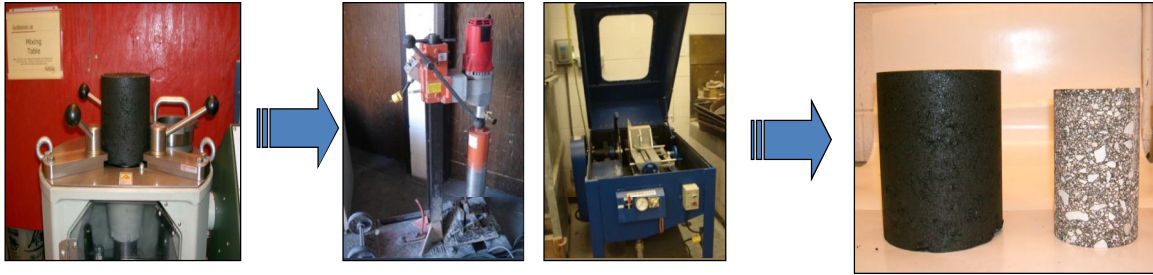
Figure 4-2. AC Specimen Production Process for the Dynamic Modulus Testing
