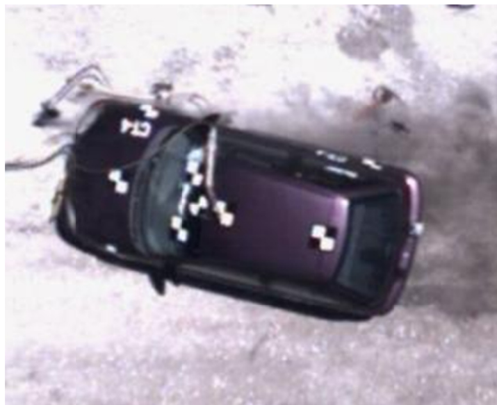
Figure 23. Geo Metro Overriding System Debris
