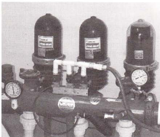
Figure 6. Photo and schematic of disc filter (schematic courtesy of Arkal Filtration Systems.)
