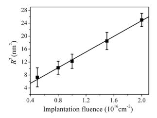
**Figure 4.**  $R^2$  versus implantation fluence f (samples 1–5), the solid line is the linear fit to the experimental data.
