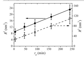
**Figure 3.**  $R^2$  ( $\bullet$ ) and  $R^3$  ( $\circ$ ) versus annealing time  $t_a$  at 600 °C (samples 3, 6–9), the solid and dashed lines are linear fits to the experimental data.
