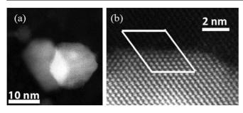
**Figure 7.** (a) High resolution TEM image corresponding to the [0 1 1] zone axis, showing the epitaxial Pb/Si interface; (b) zoom in of the Pb/Si interface, the Burgers circuit indicates the presence of a misfit dislocation.
