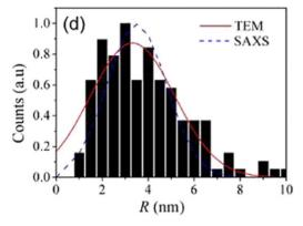
**Figure 2.** (*a*) Cross-sectional TEM image, (*b*) A vortex rendering of the 3D reconstruction of the volume showing the spherically shaped Pb NPs and a 2D Pb layer, (*c*) A slice through the 3D reconstructed volume and (*d*) size distribution histogram obtained from the TEM data of sample 3, the solid lines compare the size distributions obtained from TEM and SAXS.
