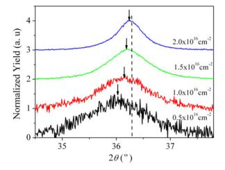
**Figure 8.** XRD  $2\theta$ – $\theta$  scans for samples with different implantation fluences after annealing, revealing a size-dependent out-of-plane tensile strain in the Pb NPs. The dashed line indicates the position of the bulk Pb (2 0 0) diffraction peak; the arrows show the peak positions for the NPs.
