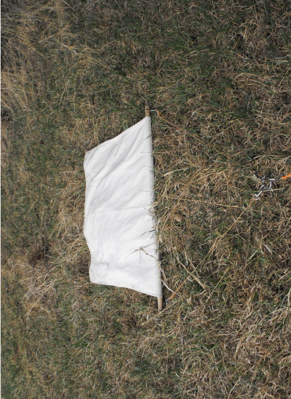
Figure 14 Tick drag made of double layered 12oz bleached denim; 1m 2 .
