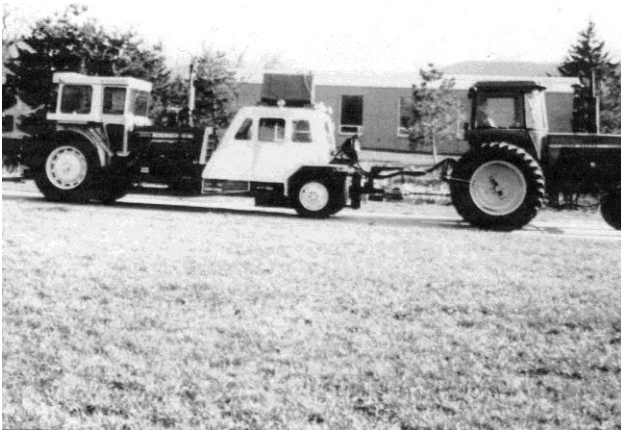
Figure 46. Test car number 4, with the Adams car mounted on an Oliver 1855 which serves as an integral load unit. The test car was now self propelled if necessary.
