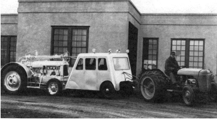
Figure 45. Test car number 3 designed by Charlie Adams in 1938, pulling a revised load tractor using the tractor engine as a compressor to provide the load..
