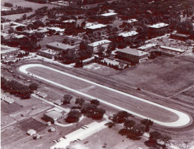
Figure 42. Concrete test track with Tractor Test Lab at left (east) end. Constructed in 1956 as a monolithic pour, without expansion joints, it improved accuracy of testing rubber tired tractors. An earth track extends around the concrete track for testing track-laying tractors.
