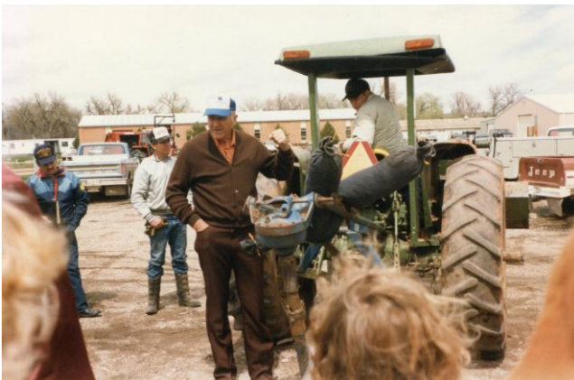
Figure 18 Schnieder demonstrating how quickly a person (the dummy called Jughead) can be trapped and killed with an unshielded power take off.
