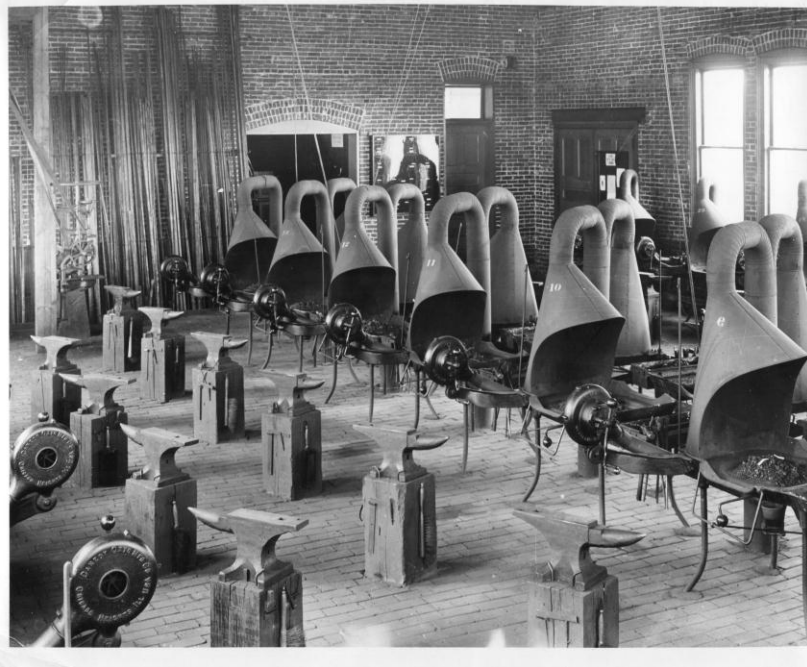
Figure 37. Forge shop in the north wing of Machinery Hall. Blacksmithing was an essential skill as machines were being introduced for farming, both for manufacturing and for repairing them .
