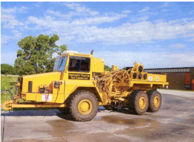
Figure 47. Test car number 5 built on a Caterpillar D300 dump truck frame. Load is provided by a hydraulic pump using four cooling fans as can be seen.
