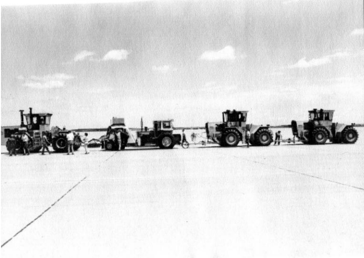
Figure 48. Steiger "Tiger" III tractor with test car #4 and 2 load units. Maximum drawbar horsepower was 356.58. Up to six load units have been used to provide draft.
