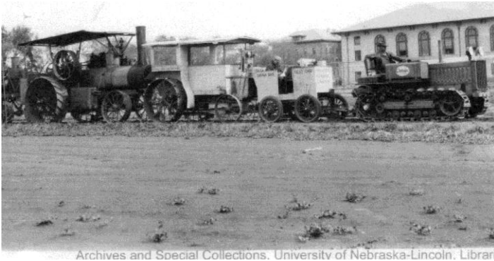
Figure 44. Test car number 2, using a load tractor which in turn is pulling a steam tractor for additional draft.
