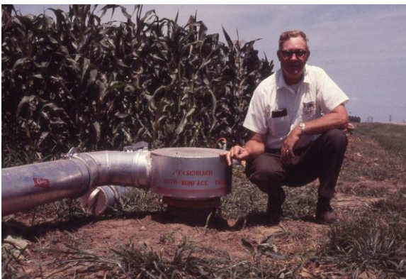
Figure 22. Fischbach and the automated gated pipe irrigation system he developed.
