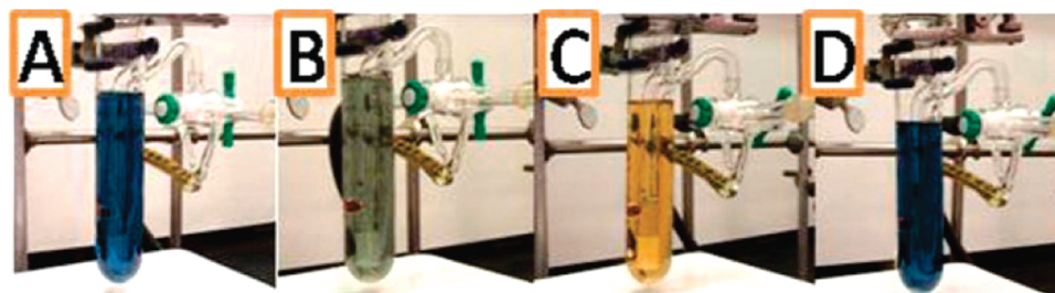
Figure 3. Reaction of 2[Rh(III)] with CO in the presence of 100 equiv of indigo carmine: (a) initial, (b) after CO introduction, (c) at reaction end point, and (d) after exposure to air.
