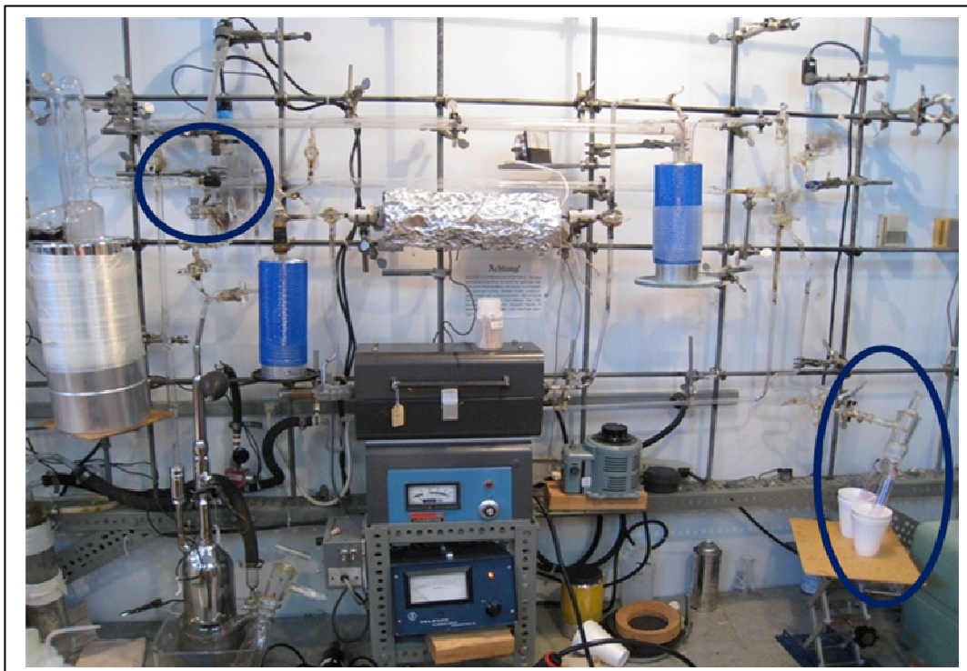
Figure S2: Experimental system for trapping of N_2 gas. When RDX was completely degraded, all gases were evacuated from the Rittenburg tube (Lower Circle) and trapped in the vacuum system except N_2 gas which was forced to the gas-tight sampling tube (Upper Circle).
