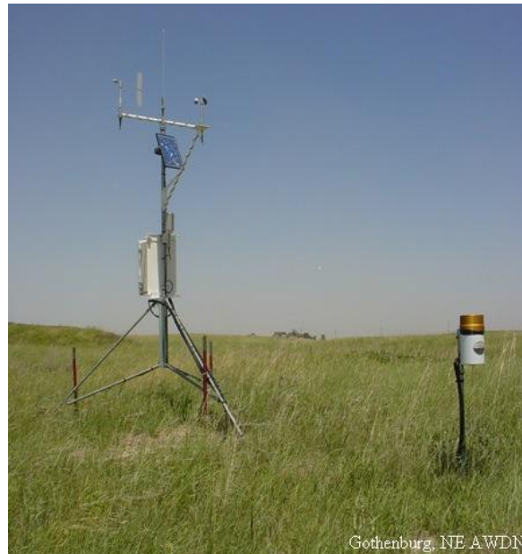
Figure 2.5. Weather station located at Gothenburg, NE. The surround grass cover is not kept at 0.12-m height. ( www.hprcc.unl.edu )
