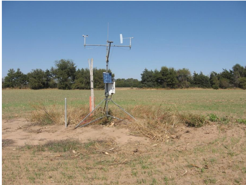
Figure 2.2. Weather station at St. John, KS. The immediate surrounding area includes a windbreak. The weather station is situated above bare ground. ( http://wdl.agron.ksu.edu/metadata.php )
