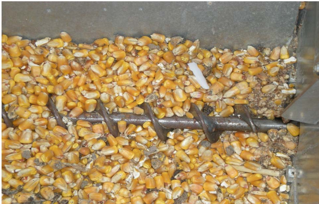
Figure 1.8. The Corn Auger in a bio furnace feeding system.
