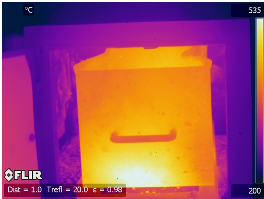
Figure 3.2. Firebox Thermal Image (°C).
