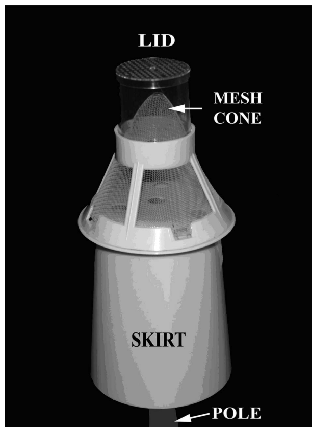
Figure 2. A photograph of a boll weevil trap with the four locations of the trap assembly labelled.
