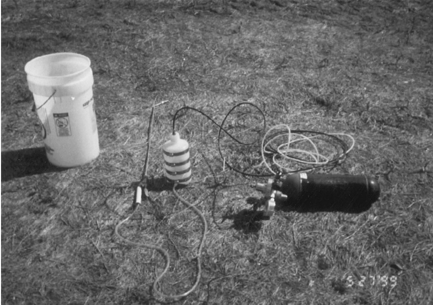
Figure 1. Equipment used for applying 15 N labeled material to microplots that do not have barriers placed around them. Included from left to right are a bucket for carrying the gas cylinder, the spray wand used for spreading the 15 N labeled material, the polyethylene bottle for the liquid that is sprayed onto the microplots, hoses and the gas cylinder that supplies the pressure.
