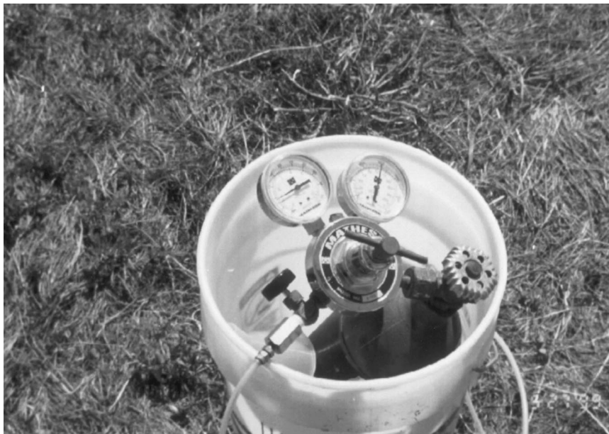
Figure 2. Gas cylinder with pressure regulator and hose for attachment to spray equipment.
