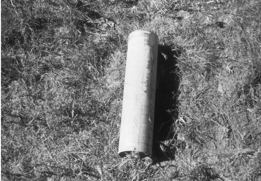
Figure 7. Single cylinder that has been removed after 10 years from a long-term grassland study of ^{15}\text{N} dynamics in Colorado. The cylinder still contains soil that will be removed in layers for laboratory analyses.
