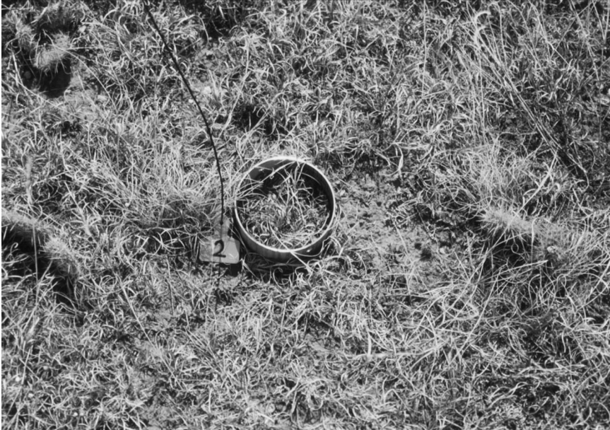
Figure 6. The top of a metal cylinder that has been placed into the soil for use in a long-term grassland study of ^{15}\text{N} dynamics in Colorado.
