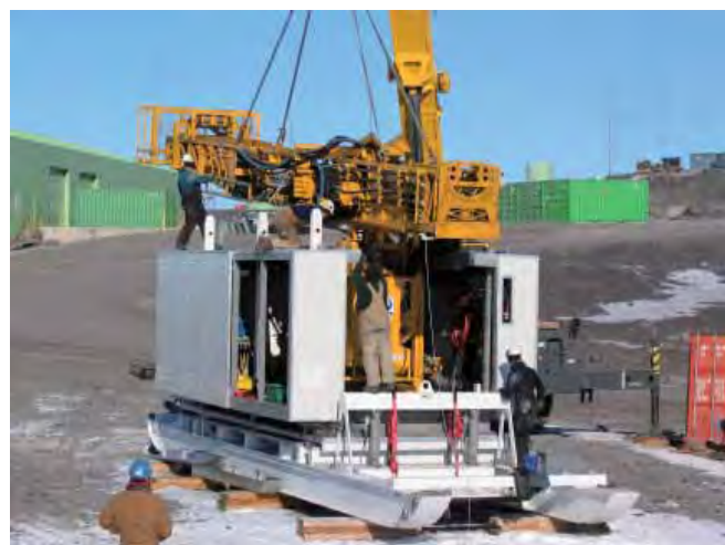
Figure 3. Attaching drilling rig mast to jack-up platform after off-load in McMurdo. Assembly of ANDRILL System at ice edge near New Zealand's Scott Base.
