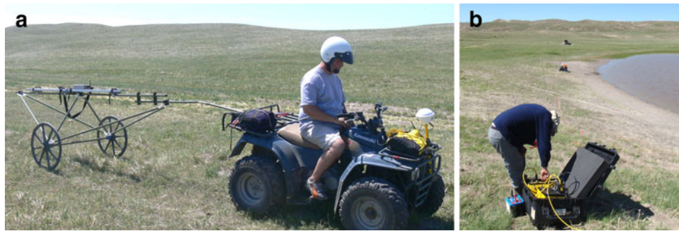
Fig. 3 Field instrumentation: a the GEM-2 is mounted on a fiberglass cart and pulled by an all-terrain vehicle (ATV); the GPS is mounted on the front of the ATV. b the eight-channel resistivity unit and switch box
