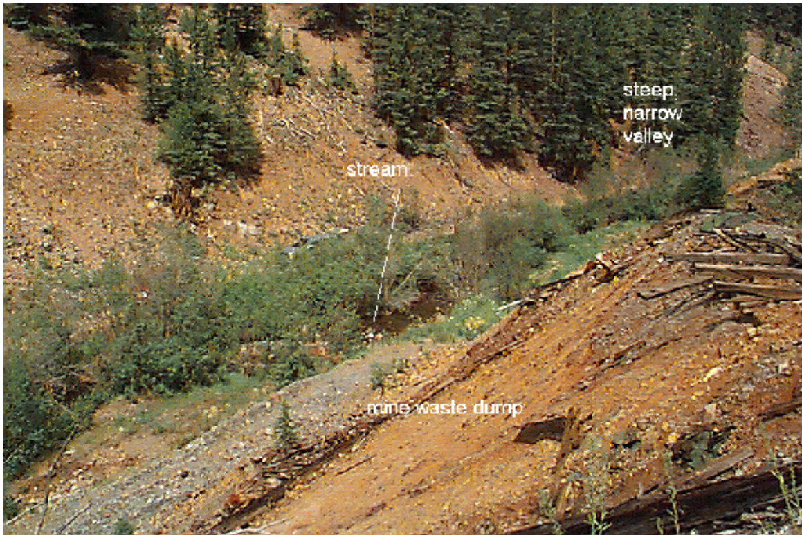
Figure 1. Typical abandoned mine waste dump in the Rocky Mountains of the western U.S. Oxidized ore and soil developed from mine waste material form a steep slope in a narrow valley drained by a perennial stream. Surface runoff from solids on the dump and infiltration through the dump contributes sediments and dissolved metals to the stream. The underground mine here exploited a tungsten skarn deposit that was last worked in 1955. Photo taken August 1999.
