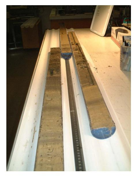
Figure 7. Photograph of core sections sampling the same stratigraphy from three parallel holes aligned for subsampling.
