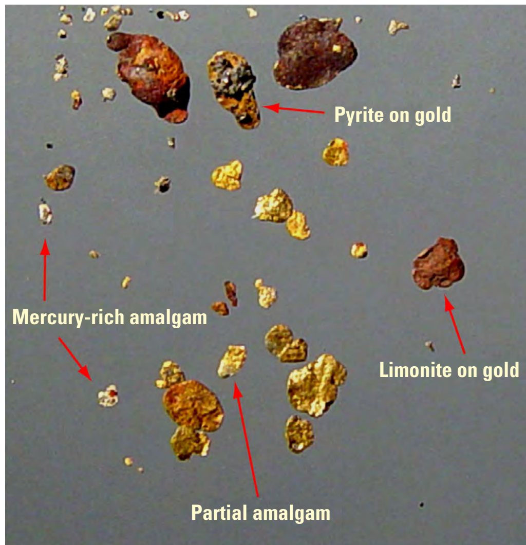
Figure 13. Gold and amalgam grains from heavy-mineral concentrate 5A from Englebright Lake, California.
