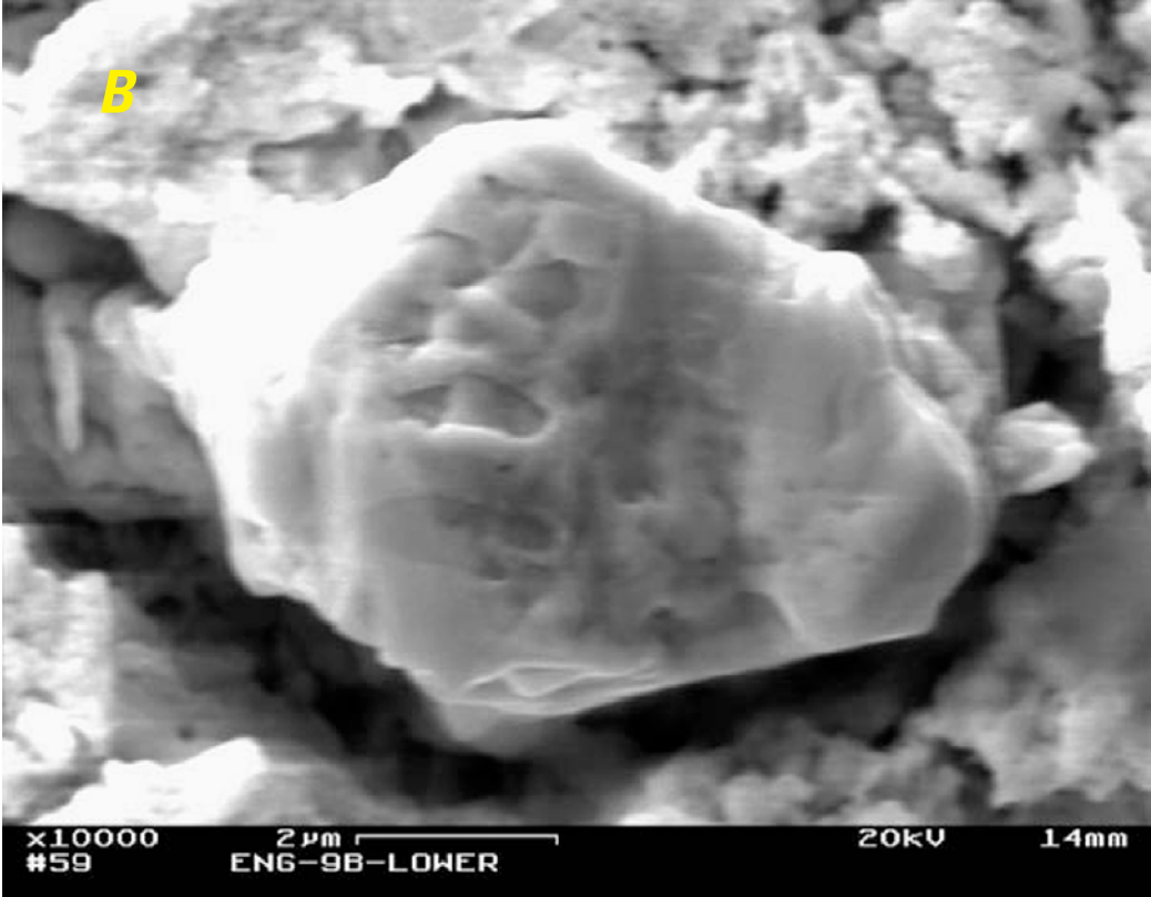
Figure D9. Amalgam grains (sample 9B) (A) Aggregate containing amalgam crystal in upper right, and (B) Close-up view of the amalgam crystal, dimensions 6 x 8 micrometers.
