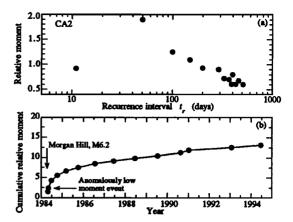
Figure 3. Data for the CA2 sequence of 14 repeating earthquakes. (a) Relative moment vs. recurrence interval. We were unable to determine  $f_c$  for the CA2 sequence, which appears to have shorter duration than CA1. Moment decreased systematically with recurrence interval for interevent times greater than 50 days. (b) cumulative moment release vs. event date showing decay of the aftershock rate to a roughly constant moment release rate.
