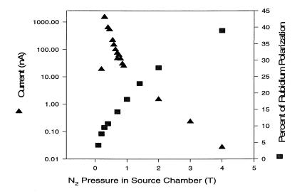
Figure 3: Current and Rubidium Polarization vs Nitrogen Pressure
