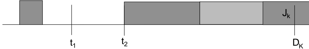
Figure 3. Instance of the SURE schedule when J_k misses a deadline at time D_k .
