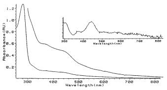
FIG. 2. **Absorption spectra of FDH.** The electronic absorption spectrum of "as isolated" FDH is shown (*lower spectrum*). The area where FeS clusters absorb is shown in the enlarged scale (*upper spectrum*). *Inset* shows the difference spectrum (oxidized enzyme minus formate reduced enzyme). The maximum in the difference spectrum is at 450 nm due to the reduction of FeS clusters. The enzyme was reduced with 10 mM formate for 5 min at room temperature.
