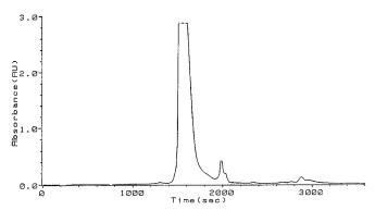
FIG. 1. **Purification of FDH on a DEAE-HPLC column.** FDH purified by phenyl-Sepharose and hydroxyapatite chromatography was further purified on a DEAE-HPLC column as described under "Experimental Procedures." Elution was followed by absorption measurements at 280 nm. The main peak eluted at 1570 s represents FDH. Minor peaks represent impurities.
