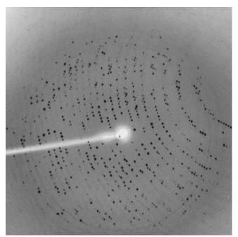
FIG. 6. A 1-degree oscillation image of a native FDH crystal. The image was taken with an R-AXIS detector at a crystal to detector distance of 175 mm and a 5-degree  $2\theta$  swing angle. The exposure time was 30 min.
