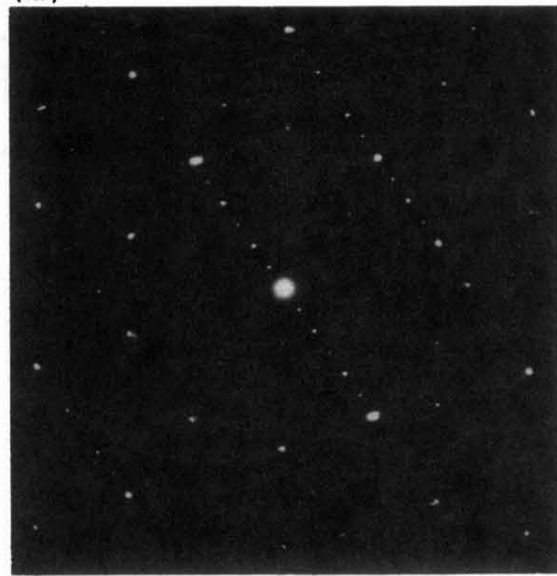
FIG. 14. SAD patterns of the cubic approximant phase along icosahedral (a) twofold and (b) fivefold directions. The directions within the cubic unit cell correspond to (a) \langle 100 \rangle and (b) irrational zone axes.
