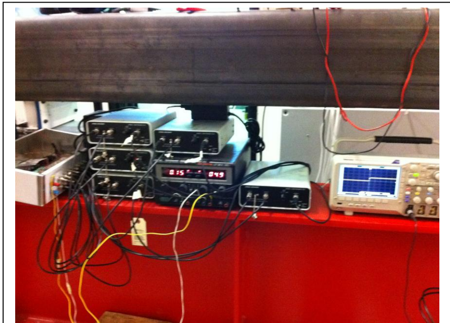
Figure 5.3.1: Part of the data acquisition system set up for the strain gages, this include the junction box, signal amplifiers, power supply and a DAQ.
