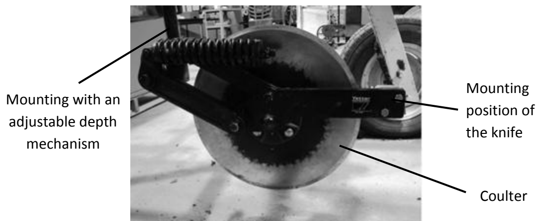
Figure 3-2: Coulter-knife assembly used to hold sensors.
