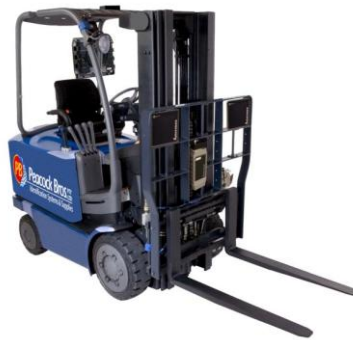
Figure 2.6. Forklift RFID reader
