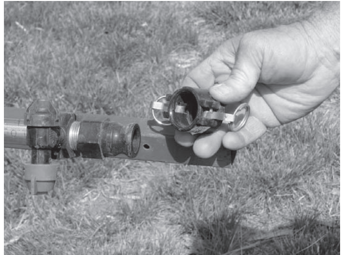
Figure 7. End cap on wet boom to drain and flush boom.
