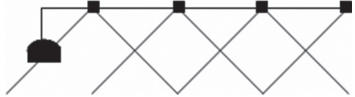
Figure 9. With a foam marker located one-half the distance between nozzles beyond the end nozzle, the marker is directly over the foam.
