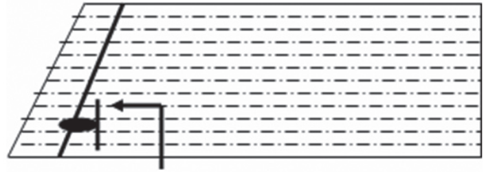
Shut off this side of boom first.
