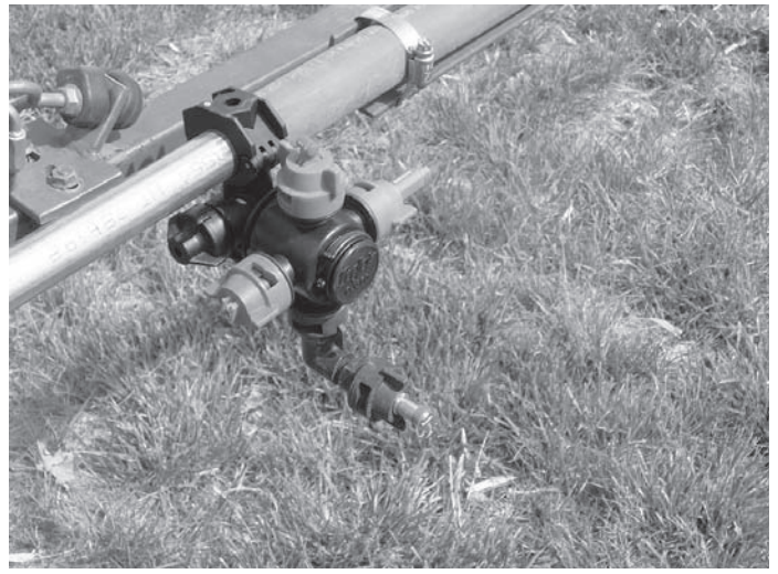
Figure 9. Multiple nozzle body on wet boom.
