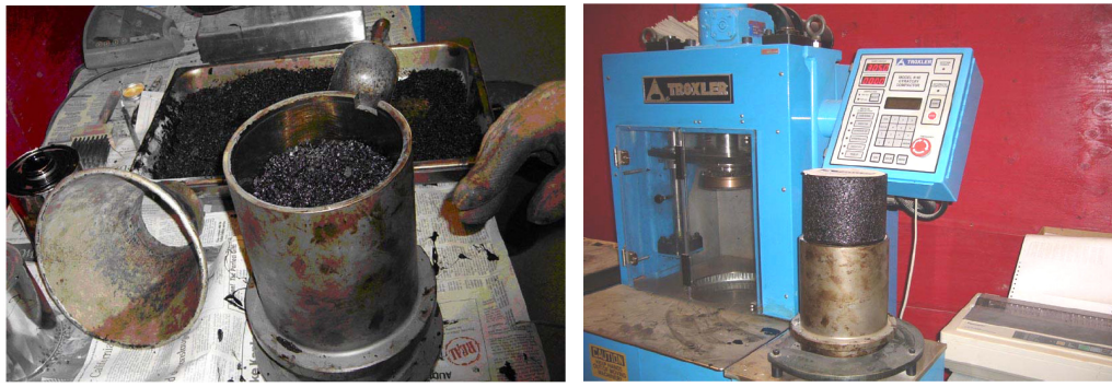
Figure 3.9 - Loose mixtures into the SGC mold and compacted HMA sample
