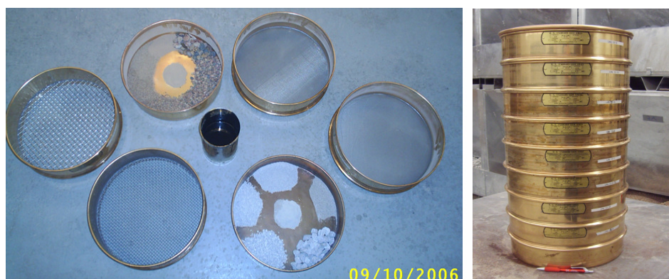
Figure 3.7 - Binder, aggregates, and sieves
