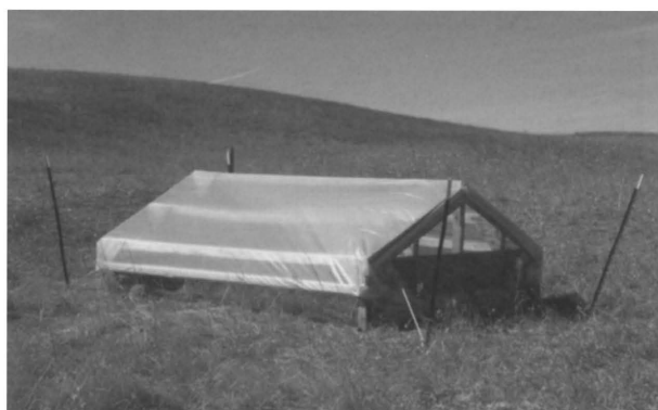
Figure 2. Wood-framed 2.5 × 3.7 × 1.2 m rainout shelters. Peaks on each end wall were covered with screening and the frame was covered with 1.5 mm polyethylene. Shelters were anchored at each corner with steel T-bar posts. These low-profile rainout shelters withstood wind in excess of 100 km hr -1 .
