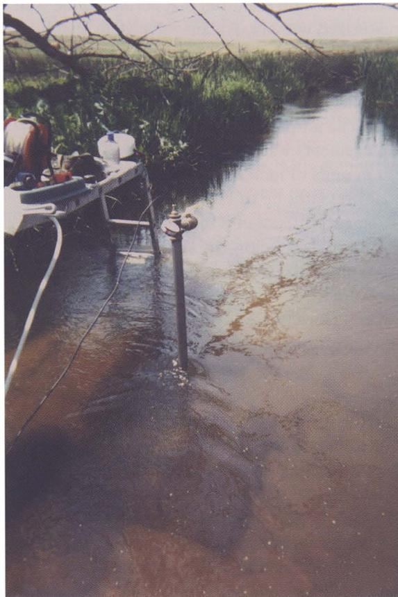
**Figure 3.** Slug-test system in use in a streambed.
