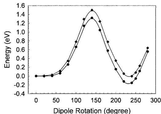
FIG. 2. The calculated total energy of a P(VDF) chain as a function of the dipole rotation around the chain axis where 0° is for the *ideal structure* and 180° for the flipping over structure. The black solid circles indicate the calculated energy and the red solid diamonds indicate the energy including the effect of the interactions. All energy values are measured with respect to the total energy of the ideal structure. The solid line guides the eyes.
