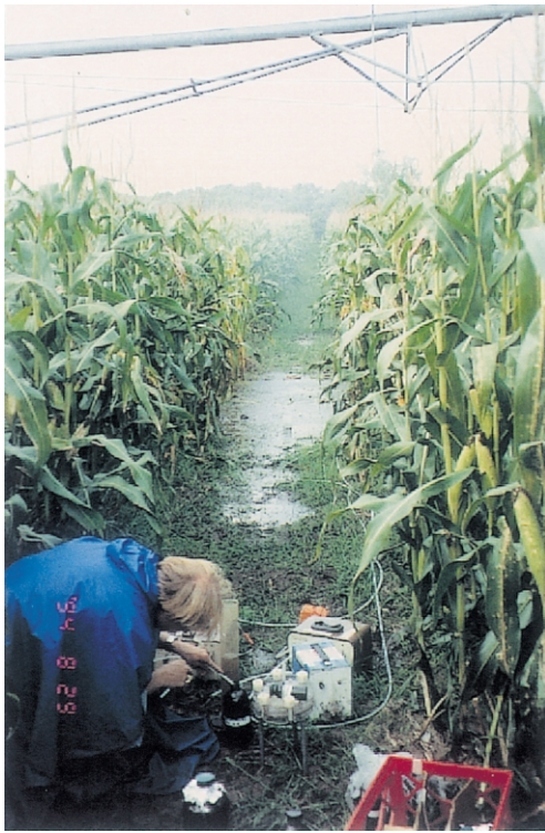
Fig. 3. Sampling run-off water ponded beneath the irrigator due to run-off. The co-author here is collecting water samples from a surface run-off collector at the lowland site. Teflon tubing extends from the collector underneath the irrigator in the background to the pump and filtration unit in the foreground.
