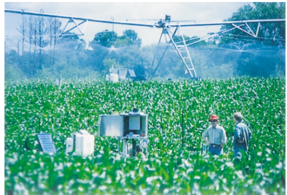
Fig. 2. View of the linear-move irrigation system applying water during a recharge experiment. The lowland site is in the foreground and the upland site in the background underneath the irrigator in this telephoto view. The two sites are approximately 78 m apart and differ in elevation by 1.4 m. The instrumentation shelters are visible at both sites.
