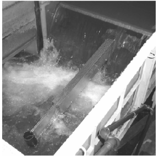
Fig. 5. Sampler assembly with collector on the downstream end of the extended center slot
