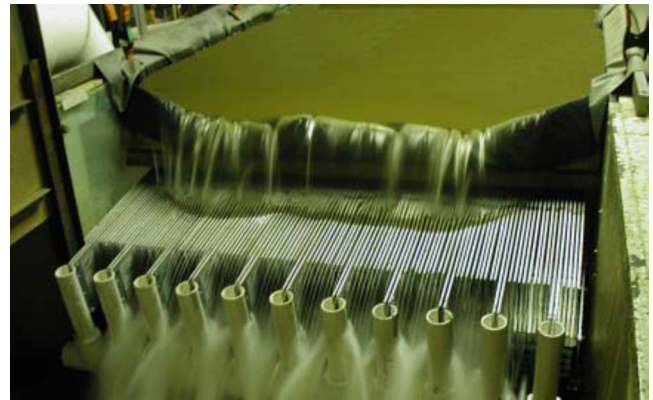
Fig. 9. Sampling assembly to test the concept of “stopped” conveyor belt system
