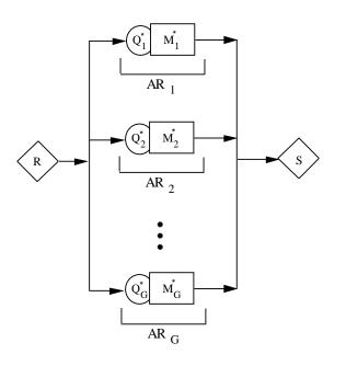
**Figure 2:** Representation of an aggregate flow line to estimate cycle time.
