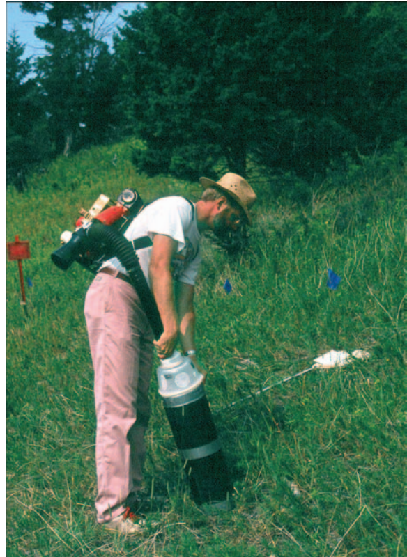
Figure 80. Backpack vacuum sampler for collecting Aphthona spp. adults, based on a modified Echo ® gasoline-powered leaf blower. Flea beetles are collected in the plastic basket attached to the vacuum hose. USDA-APHIS.
