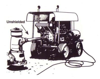
Electric power units should be de-energized before beginning any work. Capacitors on electric motors can hold a charge even though electricity is turned off. Treat them as you would a fully charged electrical system. If you suspect a short circuit as a result of feeling a "tingle," do
