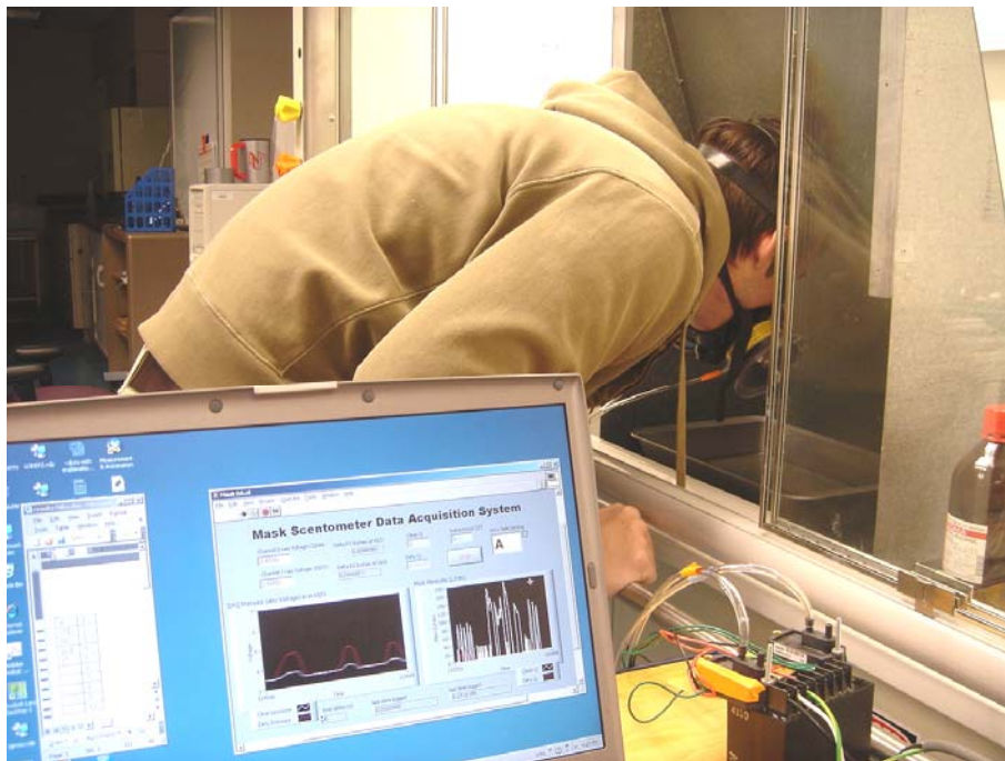
Figure 6. Experimental setup for flow measurement through the Mask Scentometer. Assessors were presented with n-butanol solutions to assess the odor dilution to threshold while airflow was measured.
