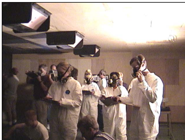
Figure 1. Odor assessors record their observations within the ISU Air Dispersion Laboratory test room.
