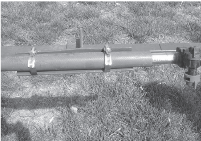
Figure 4. The bracket to hold the wet boom. The rubber hose protects the boom and the stainless steel hose clamps hold the wet boom in place.
