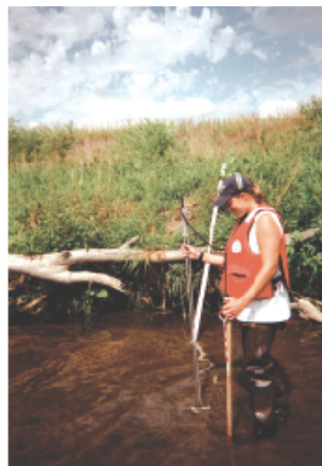
Brenda Woodward, USGS field assistant, measures flow velocity for physical habitat characterization of Maple Creek.
