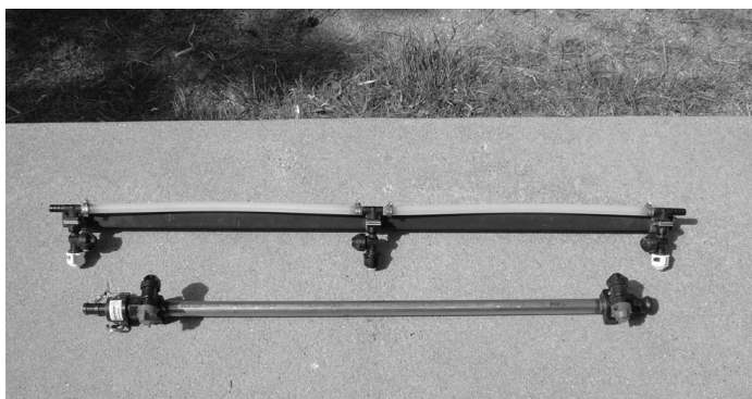
Figure 1. Sections of two booms — dry boom on top, wet boom on bottom.
