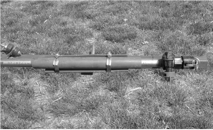
Figure 2. Angle of boom can be changed by rotating the boom within the clamps.
