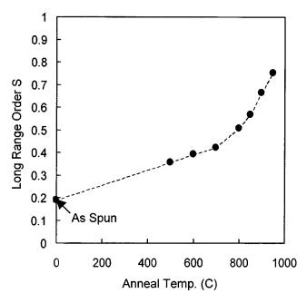
FIG. 2. Long-range order parameter S as a function of annealing temperature for the  $\rm Sm_{11}Fe_{89}$  alloy (circle).
