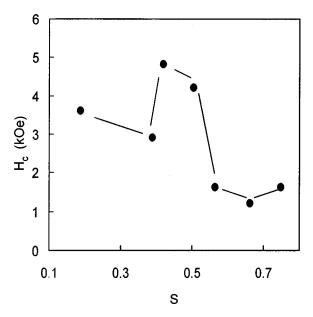
FIG. 3. Coercivity as a function of long range order parameter S for the  $Sm_{11}Fe_{89}$  alloy (circle).
