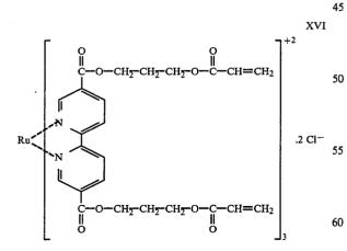
The compound of structure XVI is recovered by rotoevaporating the solvent therefrom and dissolving structure XVI is purified by chromatography on silica gel eluting wth 50% (v/v) acetonitrile in water solution saturated with KNO3. The compound of structure XVI is identified as such by visible spectroscopy and NMR spectroscopy.
