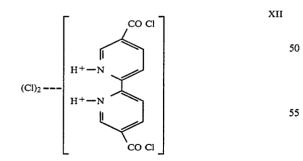
1,3 Propanediol (25 ml.) is then added to the flask <sup>60</sup> containing the acyl chloride of structure XII, and the system is then heated at 100° C. for about 30 minutes under nitrogen. The resulting solution is cooled and stored under nitrogen overnight. The solution was essentially a solution of a compound having the following structure
