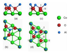
**Fig.6** Interface structure of the  $Co/Al_2O_3/Co$  MTJ for model 1 (a, b) and model 2 (c, d). Panels (a) and (c) show "front" views from a direction normal to the 3-fold axis; panels (b) and d) show "top" views along the 3-fold axis. There are two types of Co and O atoms at the interface for model 2: three O(I) atoms, one O(II) atom, one Co(I) atom, and three Co(II) atoms per unit cell. After [26].
