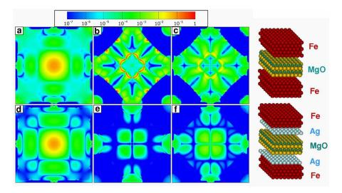
**Fig.9** Conductance (in units of  $e^2/h$ ) as a function of  $\mathbf{k}_{\parallel}$ . (a)-(c): Fe/MgO/Fe junction with 4 MgO MLs; (d)-(f): Same junction with Ag interlayers. (a), (d): Majority spins; (b), (e): Minority spins; (c), (f): Each spin channel in the antiparallel configuration. After [27].
