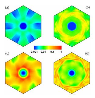
**Fig.8**  $\mathbf{k}_{\parallel}$ -resolved conductance per unit cell area in a logarithmic scale in units of  $e^2/h$  for Co/Al<sub>2</sub>O<sub>3</sub>/Co tunnel junctions with different interface structures: (a) model 1, majority spin; (b) model 1, minority spin; (c) model 2, majority spin; (d) model 2, minority spin. After [26].
