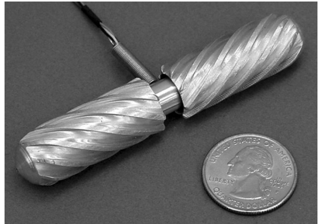
Fig. 1. In vivo wheeled robot prototype is 15 mm in diameter and 85 mm long. Here it is shown with a tether to supply power.
