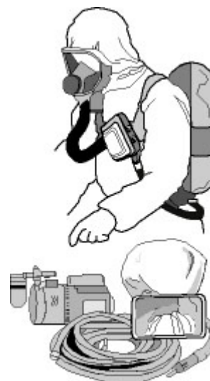
Figure 2. Self contained breathing apparatus (SCBA) with a cylinder air supply (top) and an air line that connects to a safe air source (bottom).
