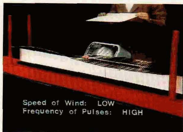
To study the collapse of the Tacoma Narrows Bridge, students can select from different scenes of an electric fan blowing on a model bridge (a). In a close-up (b) they can watch the motion of a toy car on the model bridge. Figure 7
