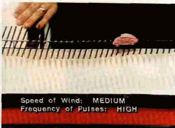
To study the collapse of the Tacoma Narrows Bridge, students can select from different scenes of an electric fan blowing on a model bridge (a). In a close-up (b) they can watch the motion of a toy car on the model bridge. Figure 7
