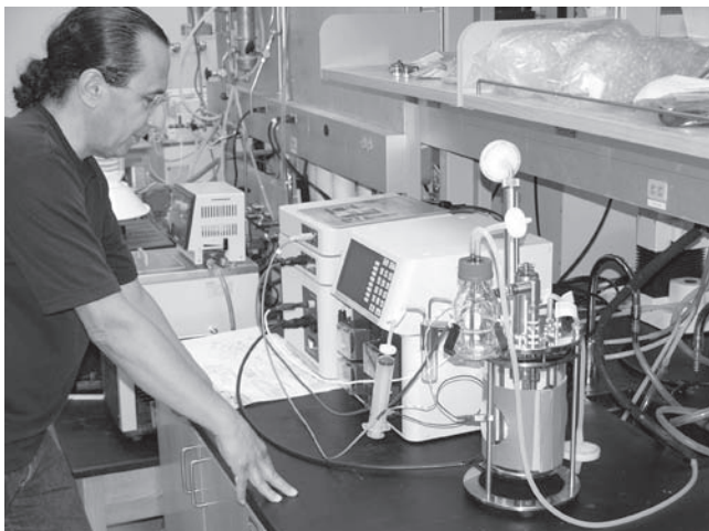
Chemical Engineer Hossein Nouredini studies adding the enzyme phytase during ethanol production, which would remove phosphorus from the organic compounds. This is just one way UNL researchers are working to reduce phosphorus in manure and in distillers grain and corn gluten feed.
